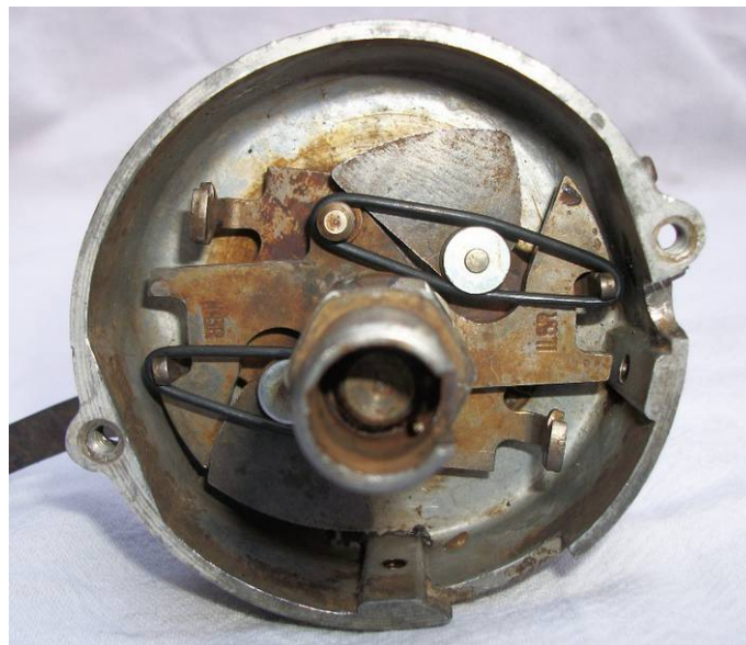
Fig. 1. Advance mechanism locked using O-rings
